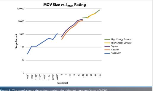
Figure 3- The graph shows the various ratings for different types and sizes of MOVs.
