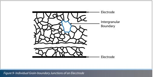
Cumulative degradation occurs as more surges or frequent voltage swells happen. In this condition, the varistor is not visibly damaged and outwardly appears functional, but it no longer offers protection. Eventually, it will proceed into a short circuit condition as the energy discharges, creating a conductive channel through the oxides.
