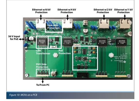
Bourns has one of the industry's most comprehensive lines of MOVs — from space-saving SMT to high energy disc and harsh environment AEC-Q compliant devices as well as the ability to offer customized MOVs.
