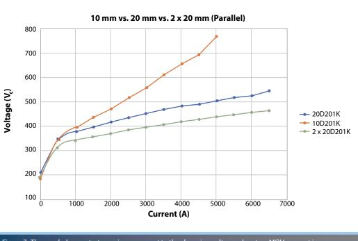
Figure 7- The graph demonstrates an improvement to the clamping voltage when two MOVs are put in parallel (green line).
