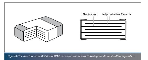
An MLV is typically offered in the 2220 size package. With an  $I_{max}$  rating of 2 kA, an MLV can easily outperform a single layer MOV in a 4032 package that is twice its size ( $I_{max}$  rating = 1200 A). Due to their small size, most MLVs are low voltage; typically rated under 200 V at 1 mA.
