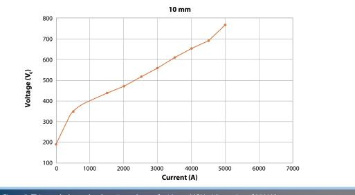
Figure 5- This graph shows the clamping voltage of a 10 mm MOV with a rating of 200 Vdc.
