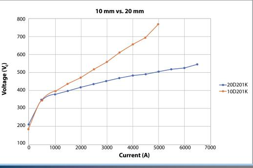
Figure 6- Shows that at 5000 A, the 20 mm disc is only clamping at approximately 500 V.
