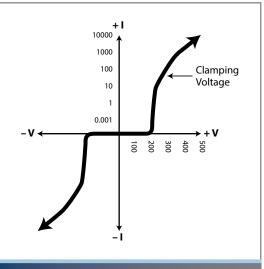
Figure 1 - This graph shows the sudden voltage clamping during a surge event that exceeds the MOV's parameters.
