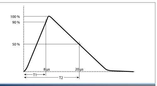
Figure 2 - For an industry standard MOV with a surge rating of 8/20 µs, the current rises to a minimum of 90 % of peak (T1) within 8 µs and 50 % of current decay at 20 µs (T2).
