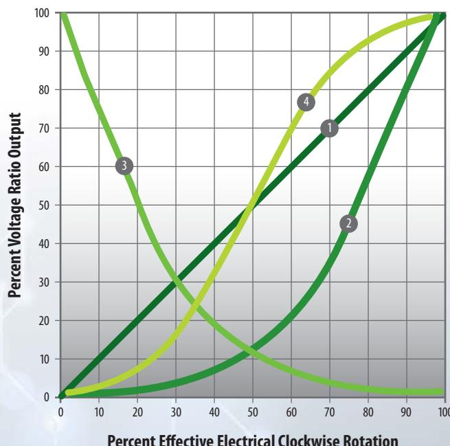
Four standard tapers have been established as shown above:
