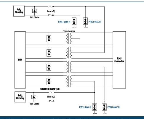
Block diagram illustration of Bourns® Model PTVS1-066-C-H in a Power-over-Ethernet (PoE) application
