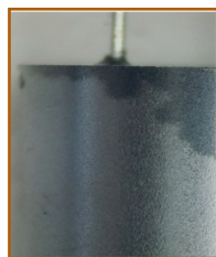
Oil Stain on Inductor Shield
