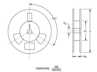
Devices are packed in accordance with EIA standard RS-481-A and specifications shown here.
