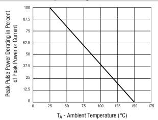
**Steady State Power Derating Curve**
