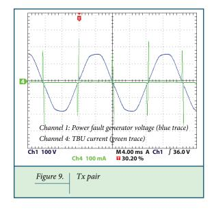
TBU™ Electronic Current Limiter GR-1089 Port Type 2 and 4 Ethernet Protection
