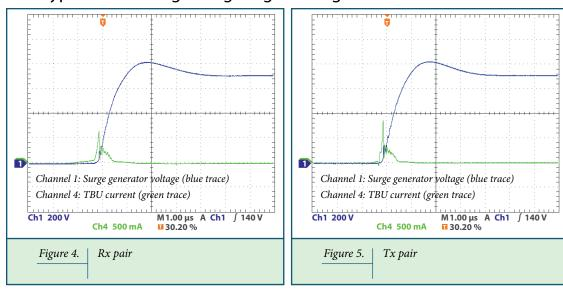
In figures 4 and 5, the generator voltage increased and the current through the TBU device caused the TBU device to trigger. The port is protected and no damage or stress occurred to the Ethernet and protection circuits; the port remains functional after the test.
