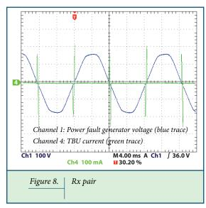
Figure 8 and figure 9 show the P850-U triggering during the power fault test. When the TBU device triggers due to a positive-going AC power fault, it protects the Ethernet port. Once the surge voltage reduces, the TBU device resets until it triggers and protects against the negative-going AC power fault. This cycle repeats for the duration of the test, fifteen minutes. No damage or stress occurred to the circuits; the port remains functional after the test.
