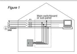
Fusing installation not required but recommended for Type 1 SPD installation according to UL 1449. Mandatory for Type 2.
